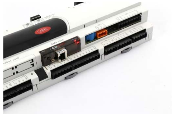
Figure 2.d - Securing pCOWeb with the cover
