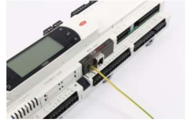
Figure 3.i – pCOWeb earth connection
