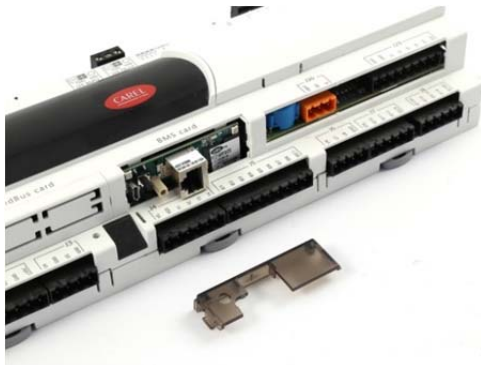
Figure 2.c - Inserting pCOWeb in the pCO controller
