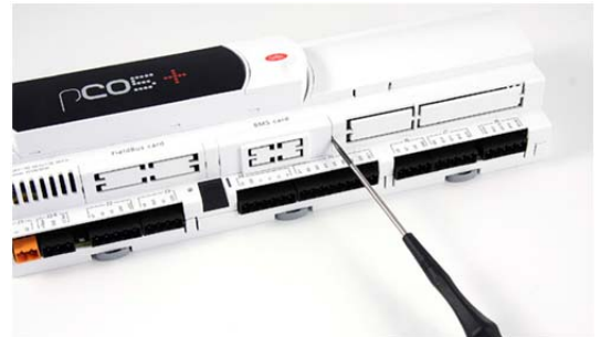
Figure 2.b - Removing the cover from the pCO controller
