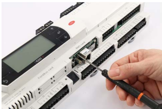
Figure 2.e - Removal of pCOWeb from controller
