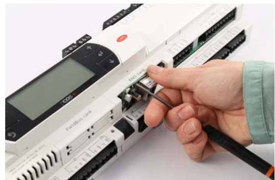
Figure 2.e - Removal of pCOWeb from controller
